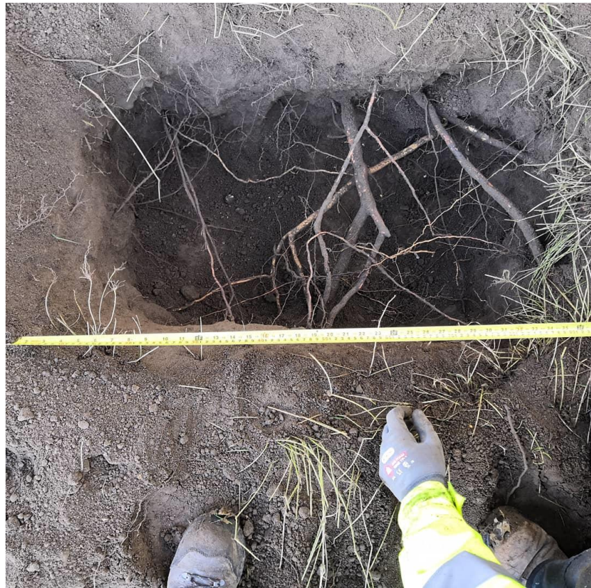
An aerial view of trial hole 2, showing a single lateral root that then subdivides into smaller diameter roots.
