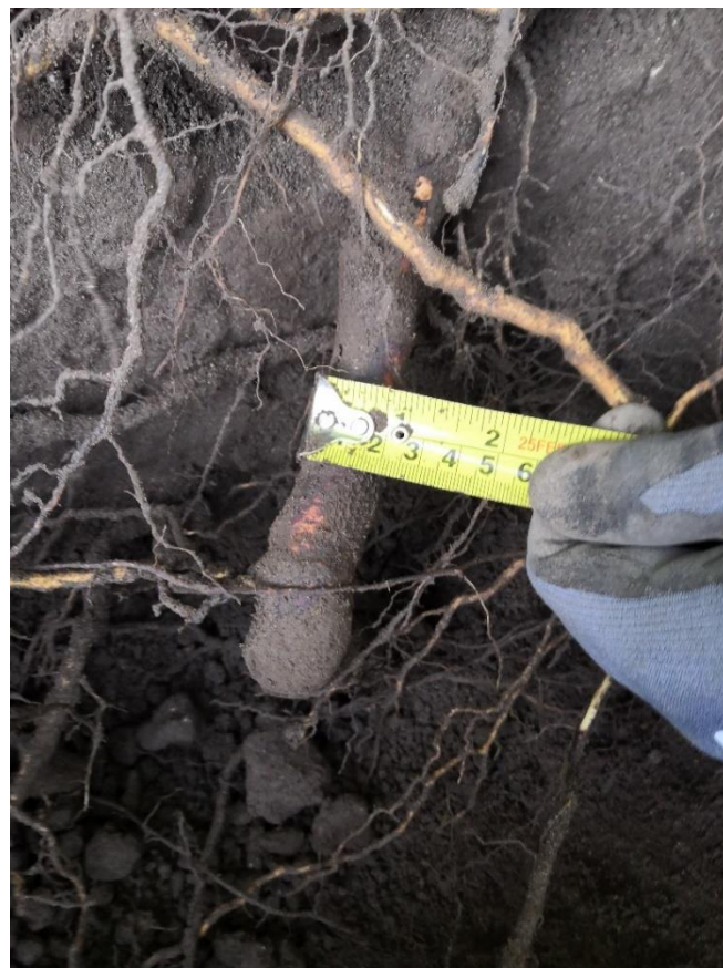
A root 22mmØ growing through a crack in the stone wall at a depth of 400mm.
